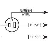
CONNECT TO A SYSTEM GROUNDING WIRE. SEE THE UNITED STATES NATIONAL ELECTRICAL CODE AND/OR LOCAL CODES FOR OTHER DETAILS AND MEANS FOR PROPER GROUNDING.
