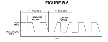
The Peak Current, Background Current, and Frequency are identical for the high energy and low energy pulses. In addition to cooling the weld down, the major effect of the low energy pulses is that they form a weld ripple. Since they occur at very regular time intervals, the weld bead obtained is very uniform with a very consistent ripple pattern. In fact, the bead has its best appearance if no oscillation of the welding gun ("whipping") is used.(See Figure B.7)
