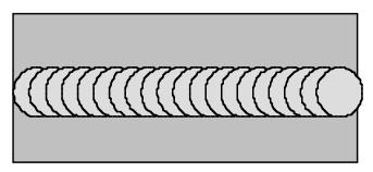
Frequency Modulation = -10 Wide weld and ripple spacing, slow travel speed.
