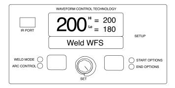
The above example shows a wire mode, constant current weld modes would show "Weld Amps" rather than "Weld WFS".
