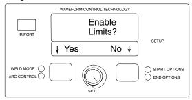
To enable or disable limits that have been established for any memory, press and hold the respective memory button in for more than 10 seconds until the Mode Select Panel displays "Enable Limits?" Pressing "Yes" will use the established limits, while pressing "No" will ignore the established limits. The limits that have been set for any memory location will not be erased if they are disabled.
