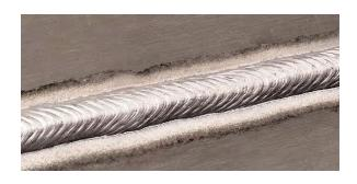
The pulsing frequency is adjustable. Changing the frequency modulation (or arc control) of the waveform changes the ripple spacing. Faster travel speeds may be achieved by using higher values of frequency modulation.
