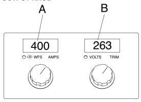
This meter displays either the wire feed speed or current value (Amps) depending upon welding process (Mode) being used and the status of the wire feeder and power source. Written below the display is "WFS" and "Amps". An LED light illuminates which value is being displayed on the meter. The knob below the meter adjusts the value displayed on the meters.
