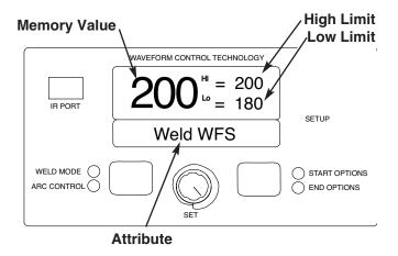
One of these four items will blink to indicate which item will change when the Mode Select Panel Knob is rotated. Initially, the selected item will be the attribute. To select the high limit, press either Mode Select Panel button and the high limit value will begin to blink. Pressing either Mode Select Panel button again will cause the memory value to blink, pressing a third time will cause the low limit to blink.
