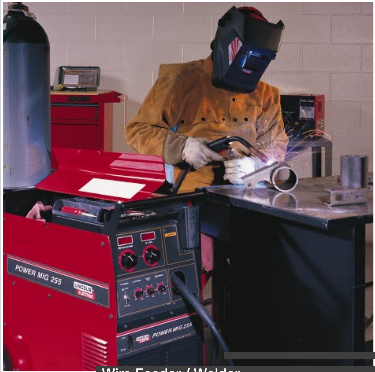
Wire Feeder / Welder
